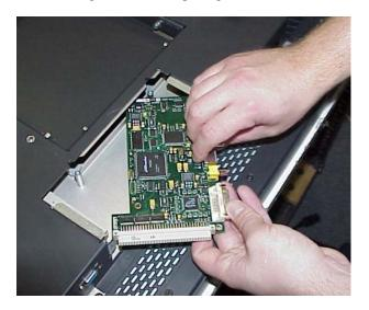
7. Align the connector on the board with the connector in the opening.
